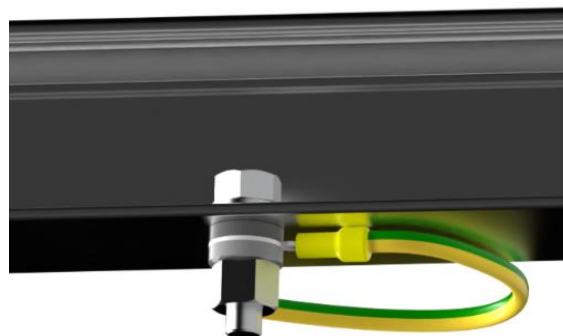
Fig. 11 Grounding of PV modules
